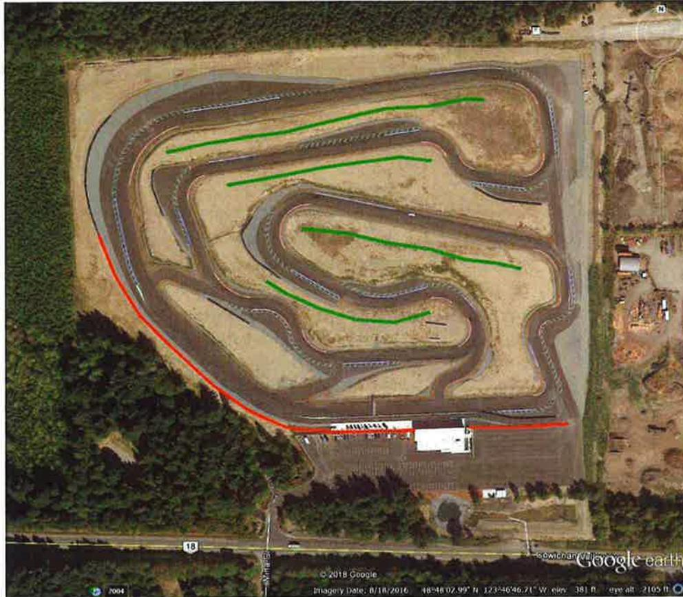
**Figure 1; Preliminary/Conceptual Locations<sup>2</sup> for Noise Barriers at VIC – Noise Wall (Red), Earth Berms or Berm/Walls (Green).**
