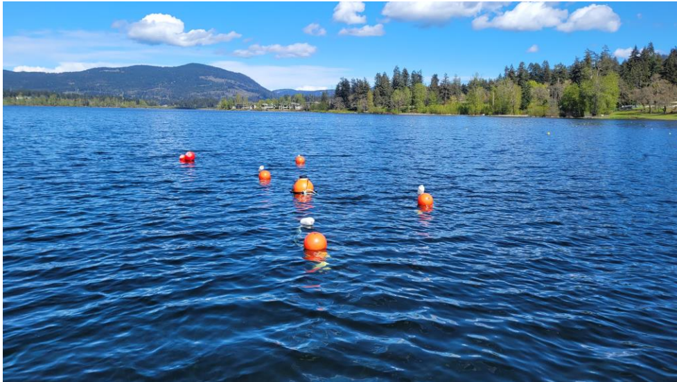
Figure 2: Photo SOD equipment deployed. Small white buoys indicate chamber locations and large orange buoy is the data logger/telemetry hub.
