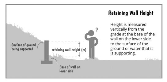
To obtain the height of a retaining wall, first determine the base location. In the above diagram, the base location of the retaining wall is at ground level where the lower side of the wall meets the ground. Then, identify the upper side where the wall meets the ground or water it is supporting. With these two points determined, take a vertical measurement between them for an accurate height assessment.
