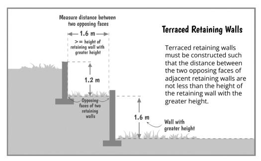
What this means is that the distance between the opposing inner sides of terraced retaining walls (measured horizontally at grade) must be equal to or greater than the height of the tallest retaining wall.
