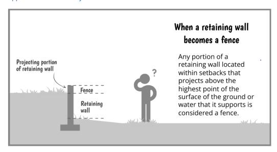
If any part of a retaining wall extends past the highest point of the ground or water it is supporting, it is a projection that is considered to be a fence.
