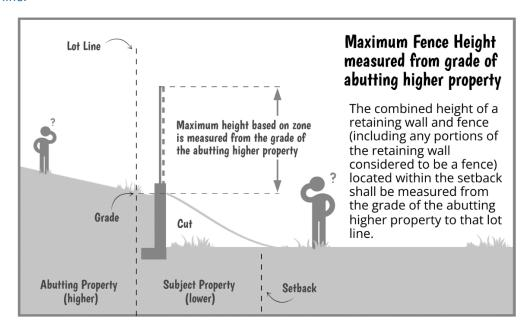
This means that when a property owner on a slope chooses to construct a retaining wall (within setbacks) along a lot line with a higher neighbouring property, the fence portion of the retaining wall is to be measured from the ground level (at grade) of the uphill neighbouring property to the top of the fence.
