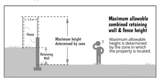
If a fence is situated directly on top of a retaining wall, the overall height of the combined structure must comply with the maximum allowable fence heights as specified in subsection 37.1(8) which speaks to fence height by zone and yard location.
