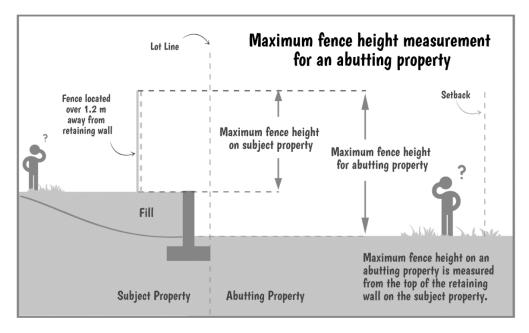
This means that if a higher elevation property owner decides to construct a retaining wall within setbacks along a shared property line with a lower neighbour, the height of the lower neighbour's fence (if located within setbacks) would be measured starting from the top of their neighbour's retaining wall to the top of their own fence.
