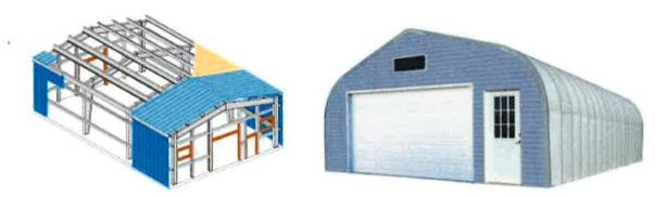
Pre-manufactured shelters and buildings are available in all sizes, materials and construction types. The smaller sizes are typically fabric covered metal or plastic frames with no foundation, these types of shelters are in most cases considered seasonal and are not designed for year round use.
