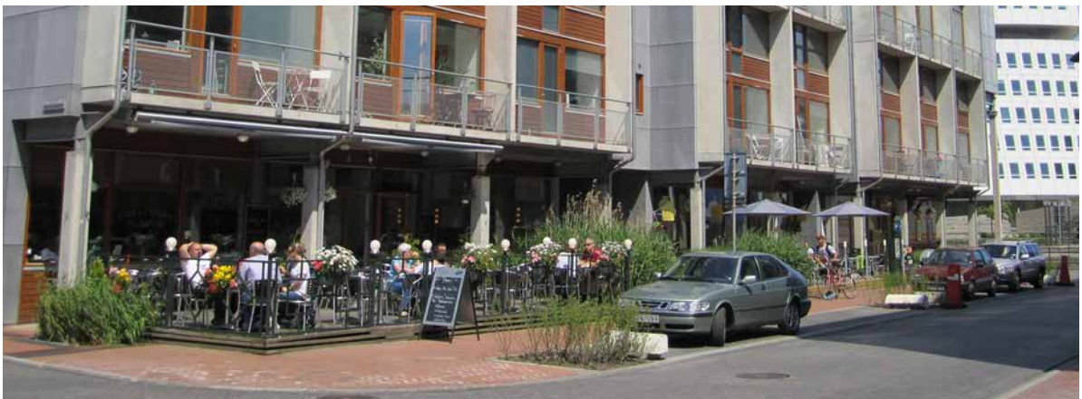
Building incorporating transparent frontage, semi-private patio, residential balconies, overhang for weather protection, and high quality materials
