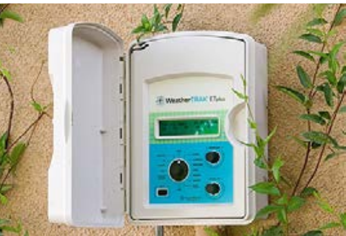
Example of a smart controller for irrigation
